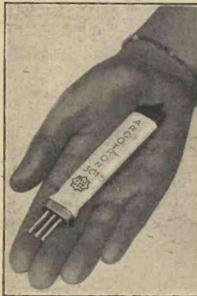
SMALLEST RECTIFIER. The Arcotron, a new type of mains valve for use in battery eliminators, recently produced by the Telefunken Company in Germany. It is screened externally by a metal covering.
