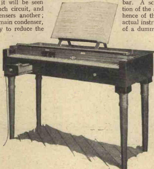
Attached to the cord over the dummy keyboard is the finger piece. Tone and volume are regulated by the controls under the left hand.
